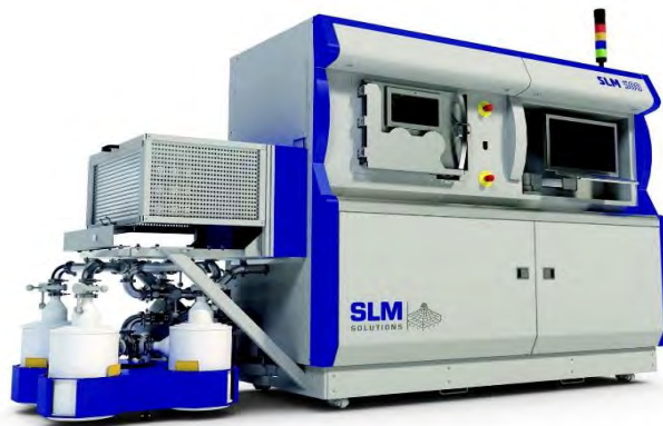
Рисунок 1.3 – SLM additive manufacturing machine.
