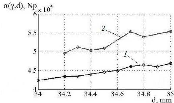
**Fig. 5.** Dependence of the signal ECT decrement on the TO diameter
