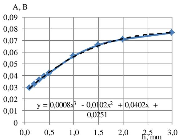
**Fig. 9.** Dependence of the maximum value of the ECT signal amplitude on the crack depth
