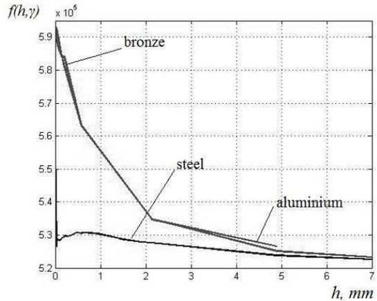
**Fig. 7.** Dependence of the ECT signal frequency on the coating thickness
