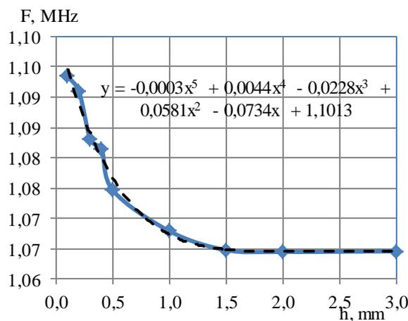
**Fig. 8.** Dependence of the ECT signal frequency on the crack depth
