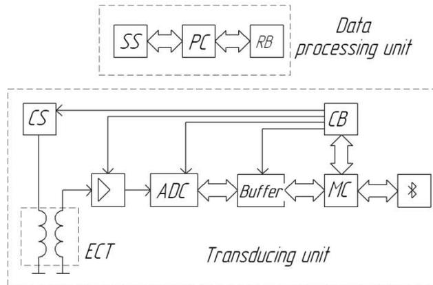
**Fig. 2.** Developed system for eddy current non-destructive testing
