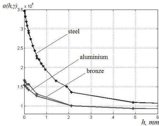
**Fig. 6.** Dependence of the ECT signal decrement on the coating thickness
