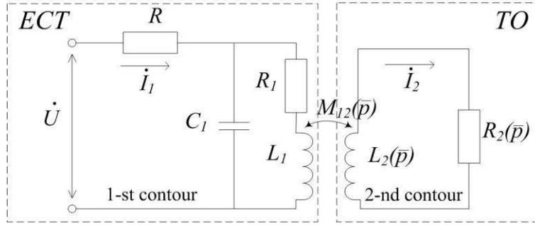
**Fig. 1.** The equivalent circuit of the system - parametric ECT and testing object
